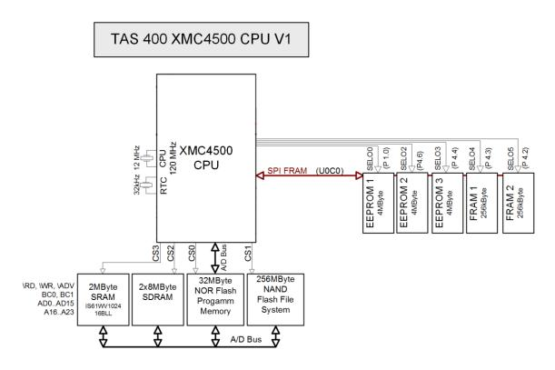
RSE-Hardware with XMC4500 / XMC4700 (Simplified Block diagram)
